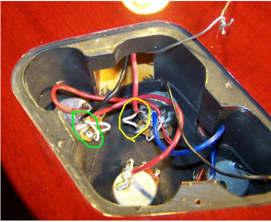
Fig. 6 Tracing the pickup wires. The bridge is in the green circle and the neck is in the yellow.
