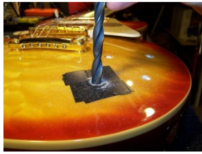
Fig. 11 3/8 drill bit by hand to finish
