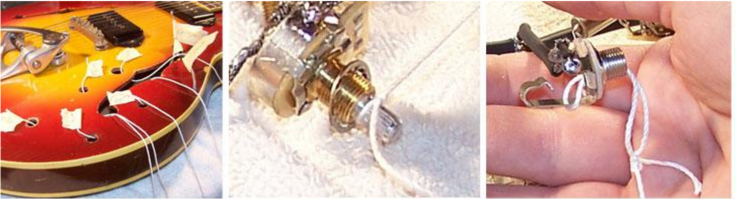
Fig. 6 Running strings for installation
