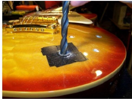
3/8 drill bit by hand to finish
