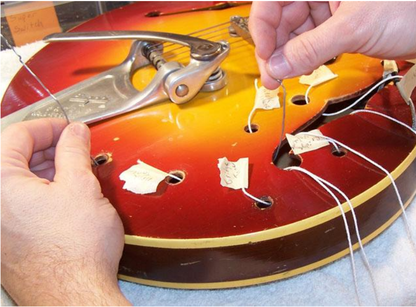
Fig. 5 Use a long piece of solder or some other material that is flexible yet has some rigidity.
