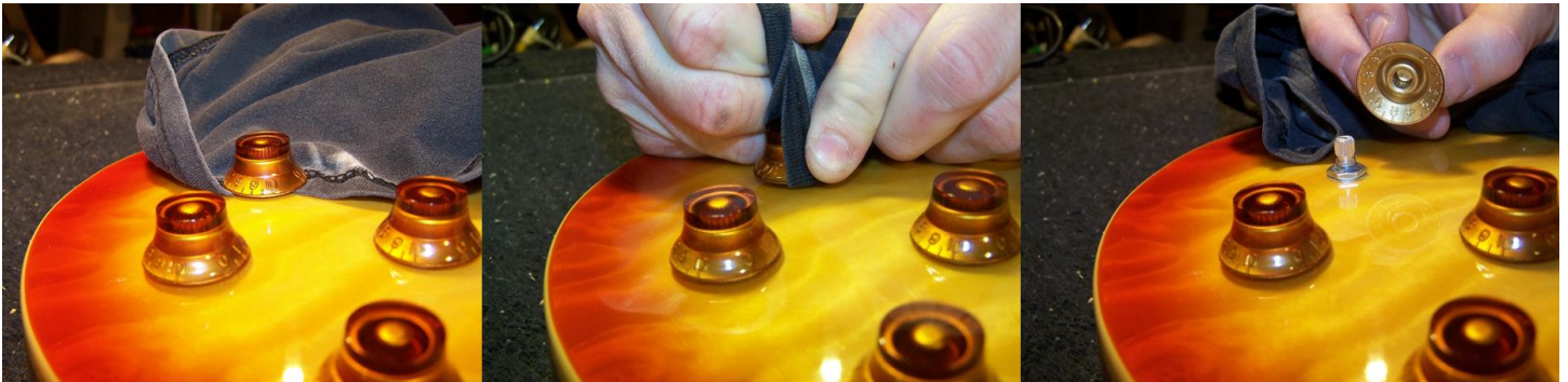
Fig. 3 Removing the knobs.
