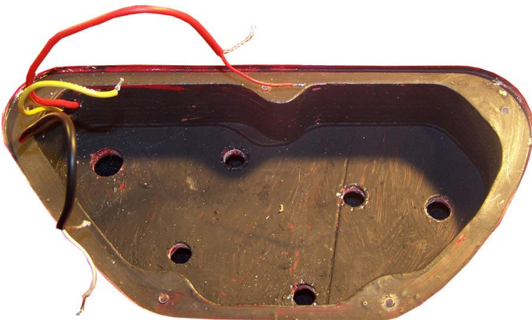
Fig.4 Old wiring removed.
