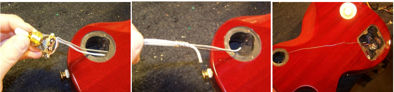
Fig. 7 Removing the old Switch and wire harness and tying off the tracing line.
