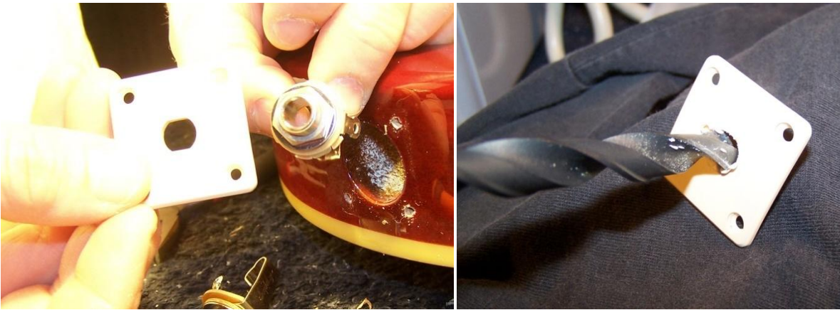
Fig. 8 Open up the jack plate so that the new jack will fit through it.
