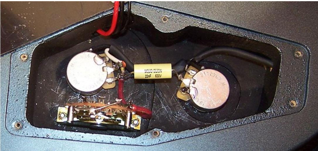
Fig.8 Kit placed in the cavity and tightened down.
