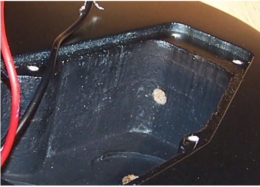
Fig.6 Open up the hole to the output jack so that the wires will fit through it.
