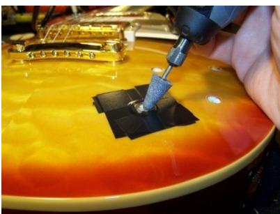
Fig. 3 Widen the top of the hole
