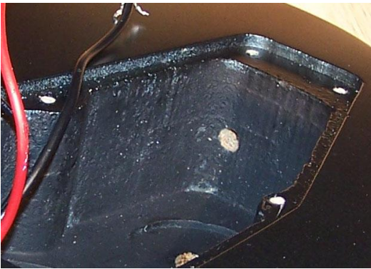
Fig.6 Open up the hole to the output jack so that the wires will fit through it.
