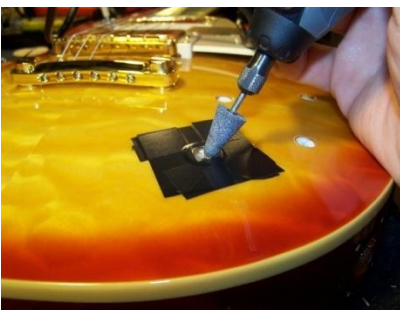
Fig. 3 Widen the top of the hole
